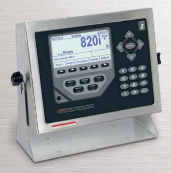
Additional features include: programmability, local/remote, configurable print/stream formats, linear 5-point calibration, truck in/out modes, batch and free-running setpoints and 16 x 350 ohm load cells per A/D card.
